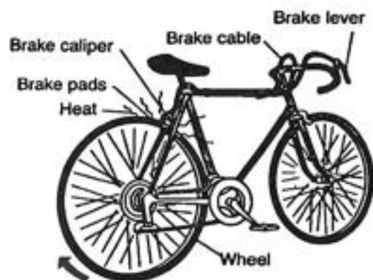
Fig. 2-6. Friction is used in stopping a bicycle. As the brake pads press against the moving wheel, mechanical energy is converted into heat energy.
