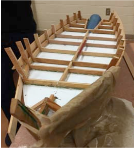
One team's ribbed boat structure being constructed.
