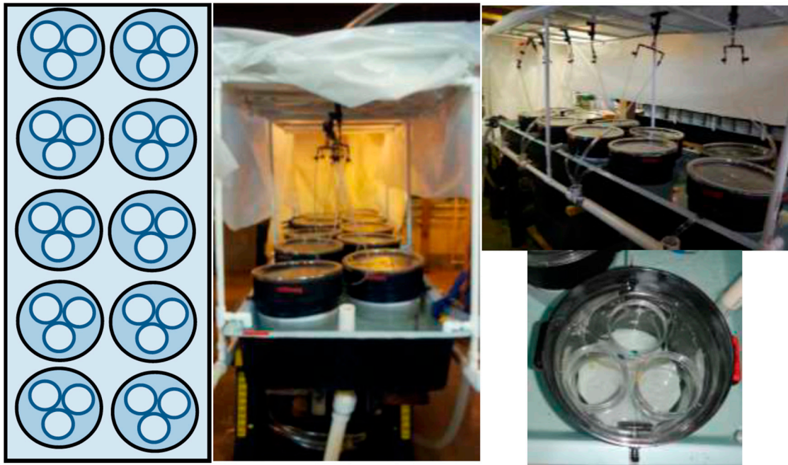
Figure 3. The LFSI 2014 system had one tank (230 × 60 cm) for each temperature (9 °C and 15 °C), ten buckets in each tank, and three small containers within each bucket in each tank. Each of the three diets were randomly assigned to the buckets and each small container randomly labeled 1 through 3. Each small container held 10 larvae, for a total of 60 larvae per diet per temperature tank.
