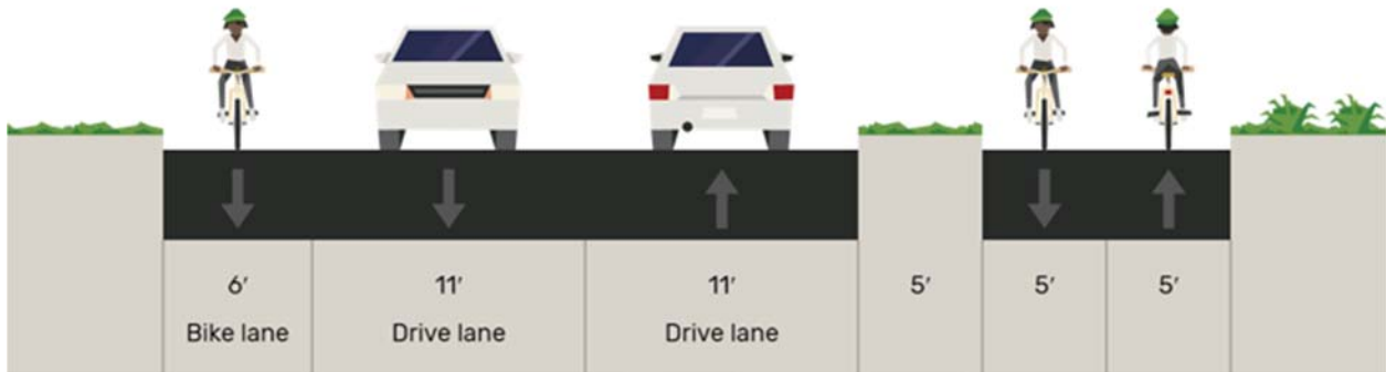
Figure 10. Cross section of Campus Backbone Drive near Clusters and McCain Drive (Proposed)
