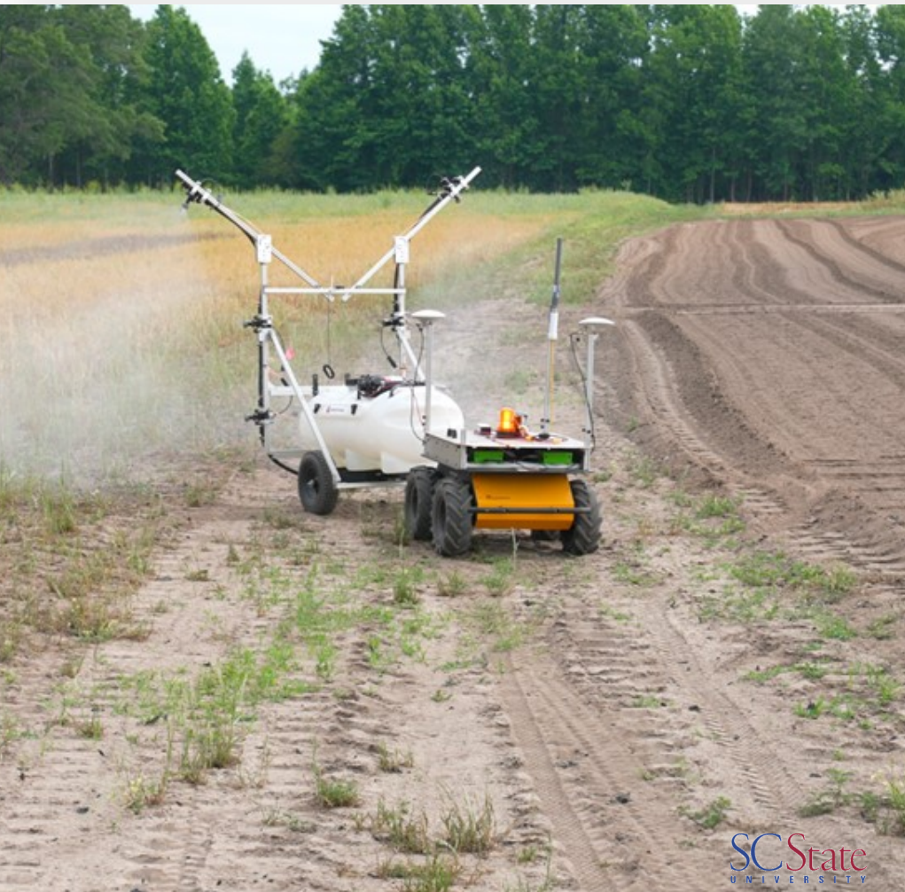
A remotely controlled defoliant sprayer conducting a spray cycle test at the SC State 1890 Research & Demonstration Farm in Olar, South Carolina.
