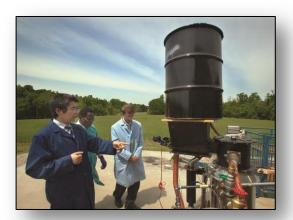
viable source of cellulosic ethanol. N.C. A&T research is showing how to convert miscanthus grass fertilized with swine waste, wood waste and municipal solid waste into syngas vapors, which, in turn are being converted to hydrogen fuels and liquid transportation fuels.
